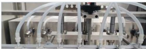
Six-Head Nozzles Visible filling path and multi-head nozzle arrangement.
