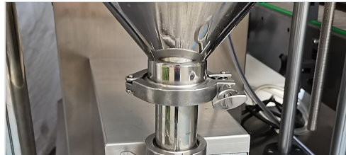
Hopper Feed Feed structure for semi-fluid or sample-based setup.
